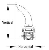
**Horizontal Clearance Required** 7" (175 mm) **Vertical Clearance Required** 19" (475 mm)
